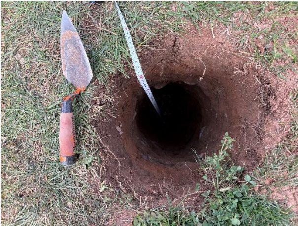
Image 11: Typical disturbed test pit
