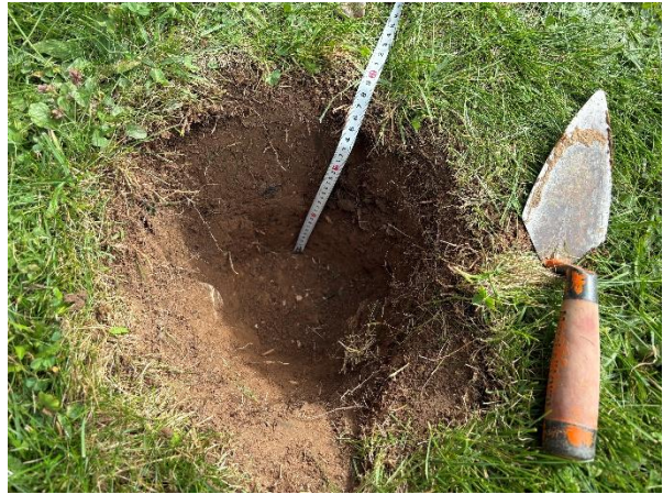
Image 12: Typical test pit
